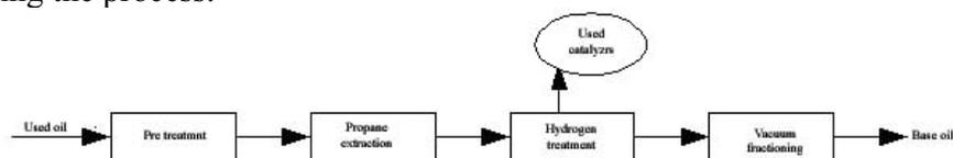
Figure 2. Schematic diagram of the NIS Refinery Belgrade used oil treatment proces
