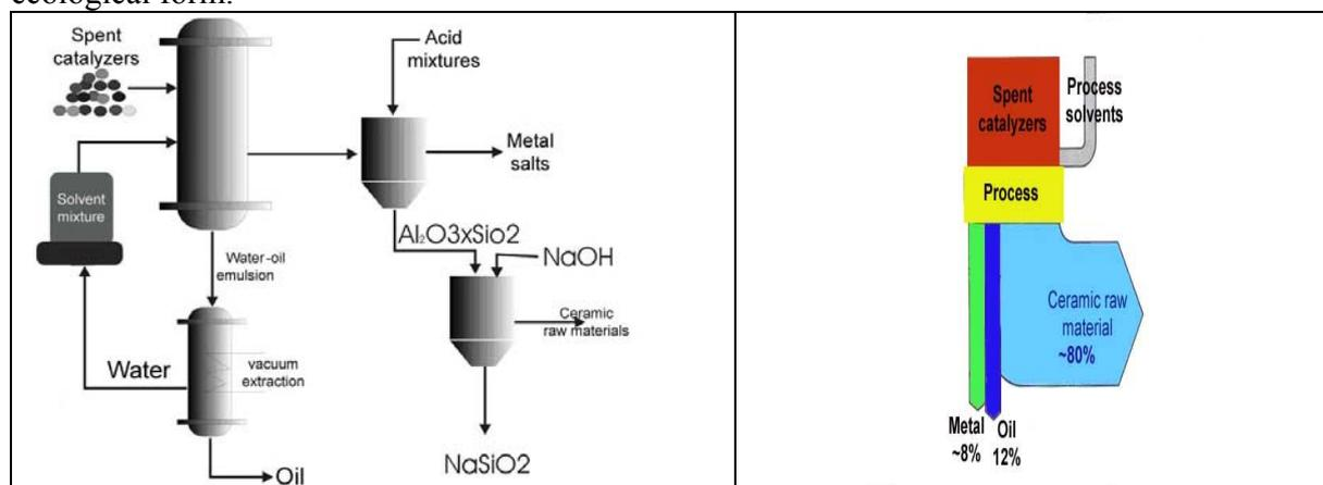
Figure 2. Scheme of oil and other organic components separation from the catalysts.
