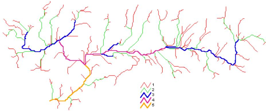
**Figure 3.** Strahler orders of the drainage reaches
