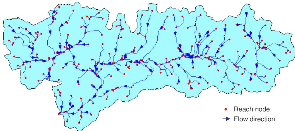
**Figure 5.** DEM-based drainage network of Küçük Menderes Basin
