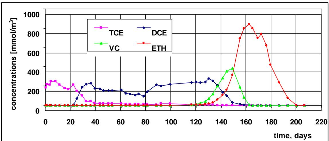
The reductive biodegradation of TCE to ETH in the bioreactor was successfully completed. Final analyses of bioreactor soil showed very low concentrations of TCE and its dechlorination products. The obtained results are presented in Table 1.
