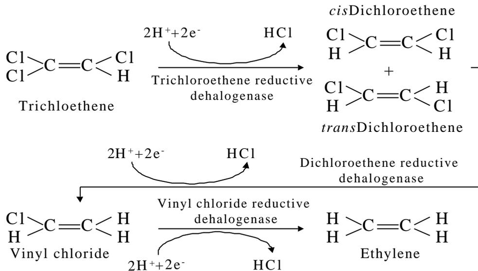
Data from the treatability study (Plaza *et al.*, 2003) provided information, which served as a basis for determining the physico-chemical and microbiological parameters for the remediation of TCE-contaminated soil in a bioreactor. It was found that bacteria present in the sludge mixture are capable of complete dechlorination of TCE to ethylene (ETH) in anaerobic conditions.
