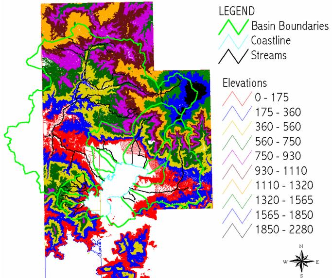
Figure 3 Elevation map obtained from GIS analyses used for hydrological calculation of Sub-basins
