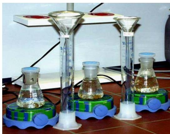
Figure 3: Photograph of percolation test equipment
