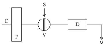
The solution (C) containing YADH and  $\text{NAD}^+$  in pyrophosphate buffer passed through the pump (P) and injection valve (V). The solution containing ethanol was injected to the stream through a valve (V). NADH absorption was used as analytical signal for conversion control.
