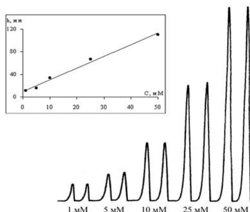
Fig.4 FIA-gramm and the dependence of the signal value of flow-injection system on the concentration of ethanol
