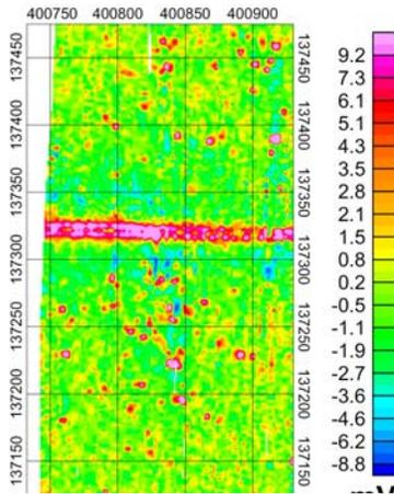
**Figure 8.** ORAGS-TEM measurements with large loop receiver at a bombing target in South Dakota, corresponding to the magnetic data shown in Figure 6. Data were acquired at 3m flight line spacing. Horizontal scale is in meters.
