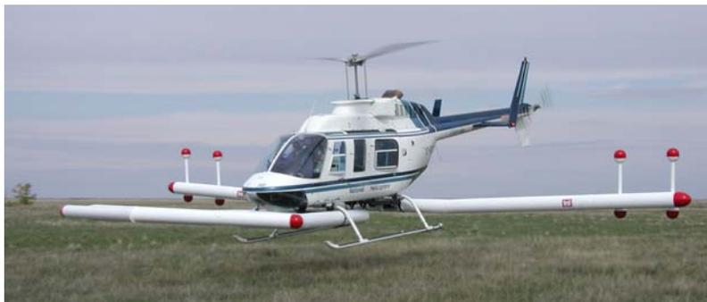
**Figure 5.** ORAGS-VG Vertical magnetic gradient system.
