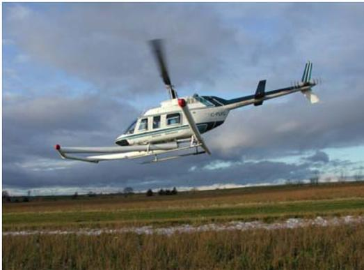
**Figure 1.** The ORAGS-Arrowhead total field magnetometer system in operation.
