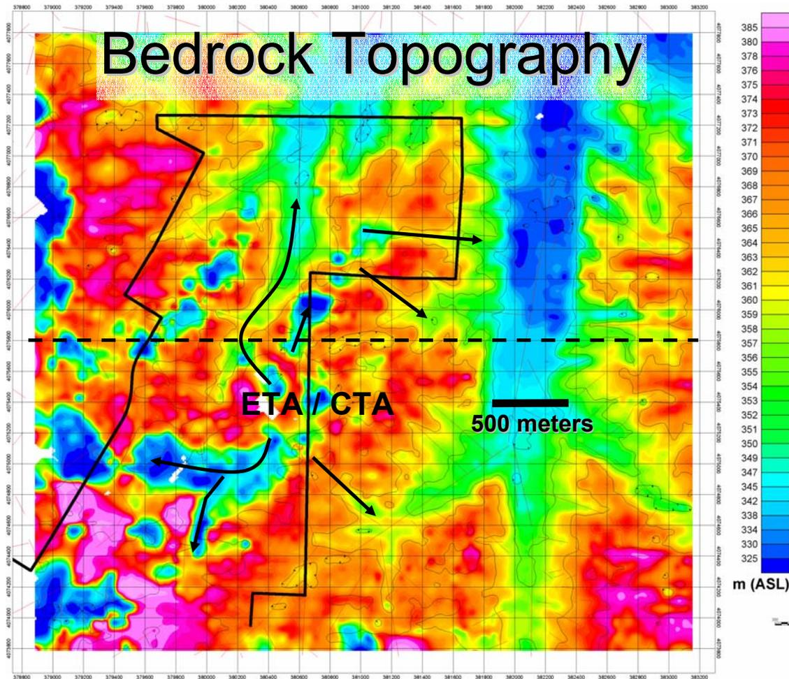
Figure 3: Bedrock topography map from airborne electromagnetic survey. Map covers area indicated as airborne survey in Figure 1. Camp Crowder boundary is shown in solid black. Dashed black line indicates airborne survey line used to correlate with the surface survey line from Figure 2. Potential contaminant pathways from the ETA site are shown as black arrows. Surface topography and photo-geologic lineaments are shown in grey.
