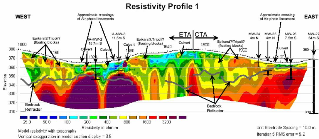
Figure 2: Surface geophysical survey results along profile 1 (as shown in Figure 1). Drilling results, seismic refractor, photo-geologic lineaments and various man-made artifacts are shown over resistivity cross-section.
