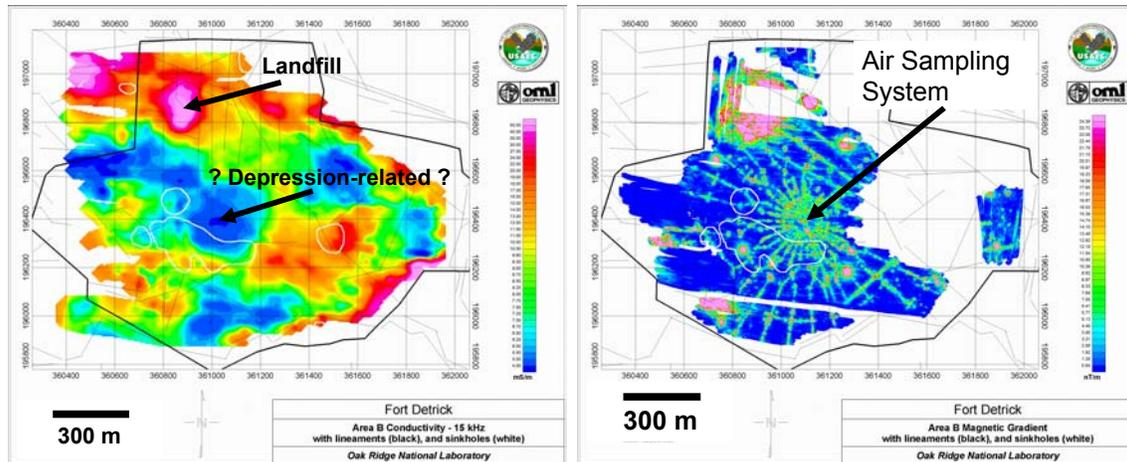
Figure 5: Apparent conductivity (left) from 15kHz airborne electromagnetic survey, and magnetic analytic signal (right) from low altitude magnetometer survey. The center of the air sampling system corresponds to the center of the conductivity low. Photo-geologic lineaments are superimposed in grey, interpreted depressions and sinkholes in white.
