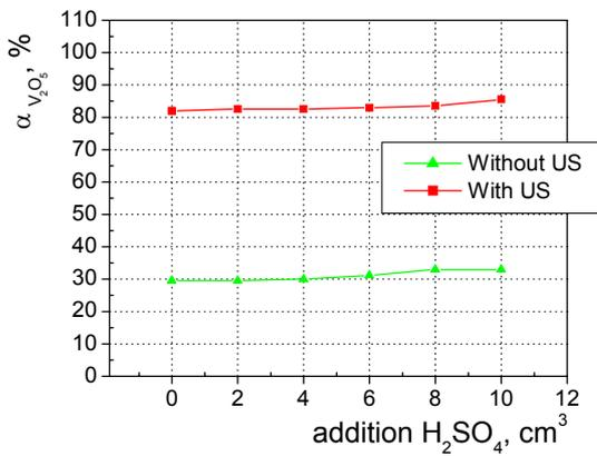
**Fig.5** Dependence of the extent of vanadium extraction on the initial sulphuric acid concentration in the extraction solution, liquid/solid phase ratio  $V_2O_5 : H_2C_2O_4 = 1 : 4$ , temperature  $T = 80$  °C
