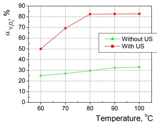
**Fig.2** Dependence of the vanadium extraction ( $\alpha_{V_2O_5}$ , %) on different temperatures, liquid/solid ratio  $V_2O_5$ :  $H_2C_2O_4$ = 1: 4,  $\square$ = 30 min
