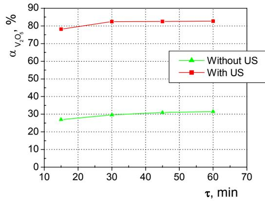
**Fig.4** Kinetic curves of vanadium extraction ( $\alpha_{V_2O_5}$ , %), solid/liquid ratio  $V_2O_5 : H_2C_2O_4 = 1 : 4$ , Temperature  $T = 80$  °C
