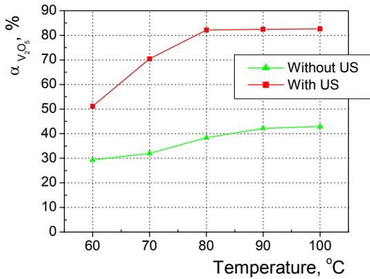
**Fig.3** Dependence of the vanadium extraction ( $\alpha_{V_2O_5}$ , %) on different temperatures, liquid/solid ratio  $V_2O_5 : H_2C_2O_4 = 1 : 5$ ,  $\tau = 30$  min
