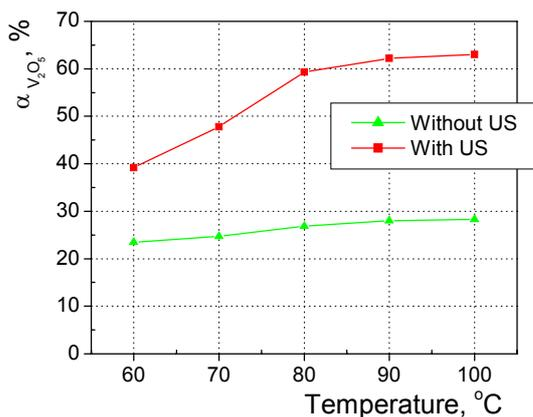
**Fig.1** Dependence of the vanadium extraction ( $\alpha_{V_2O_5}$ , %) on different temperatures, liquid/solid ratio  $V_2O_5$ :  $H_2C_2O_4$ = 1: 3,  $\square$ = 30 min
