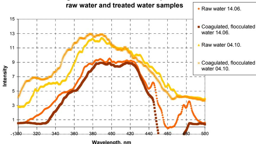
**Fig.5: Fluorescence emission spectra of the hydrophobic fractions of raw water and treated water samples**
