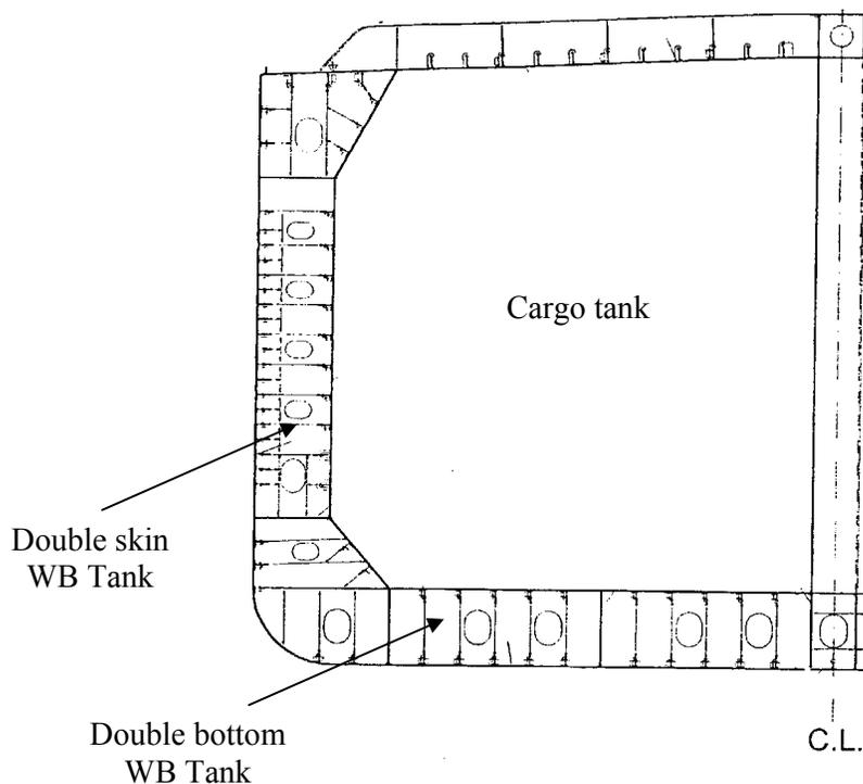
Flow-in-flow-out tanks are such tanks to which sea water is entering and exiting simultaneously and continuously during navigation, through specially performed hull openings, as to ensure the pressure at inlet opening of each tank is greater from the pressure at the outlet opening, while ensuring water flow in direction contrary of navigation course. In the starting moment, when ship is empty they are opened and the water is flooding tanks. The ship is losing displacement while increasing the
