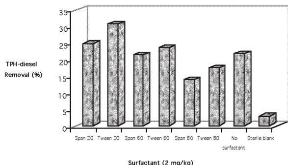
**Figure 2. TPH-diesel removal for Span and Tween single surfactants.**
