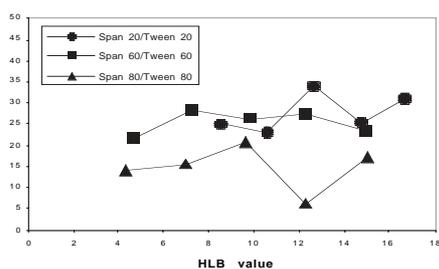
**Figure 3. TPH-diesel removal as a function of HLB value for the three surfactant families.**
