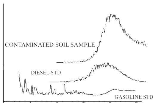
Figure 1. Contaminated soil chromatogram.
